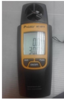
Figure 5. Anemometer for wind speed
