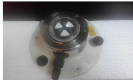
Figure 4. A pyranometer for sunlight radiation
