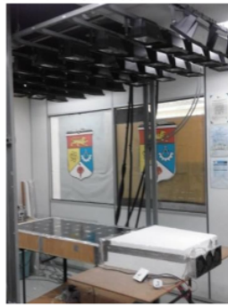
Figure 1. Indoor experimental of PVT with and without \nabla -absorber
