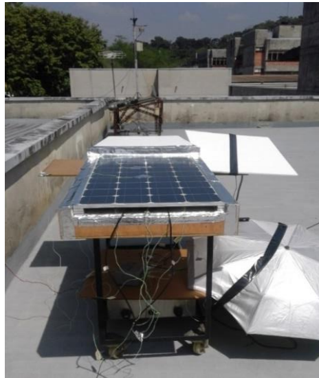
Figure 1. experimental with indoor investigation of PVT system air solar collector
