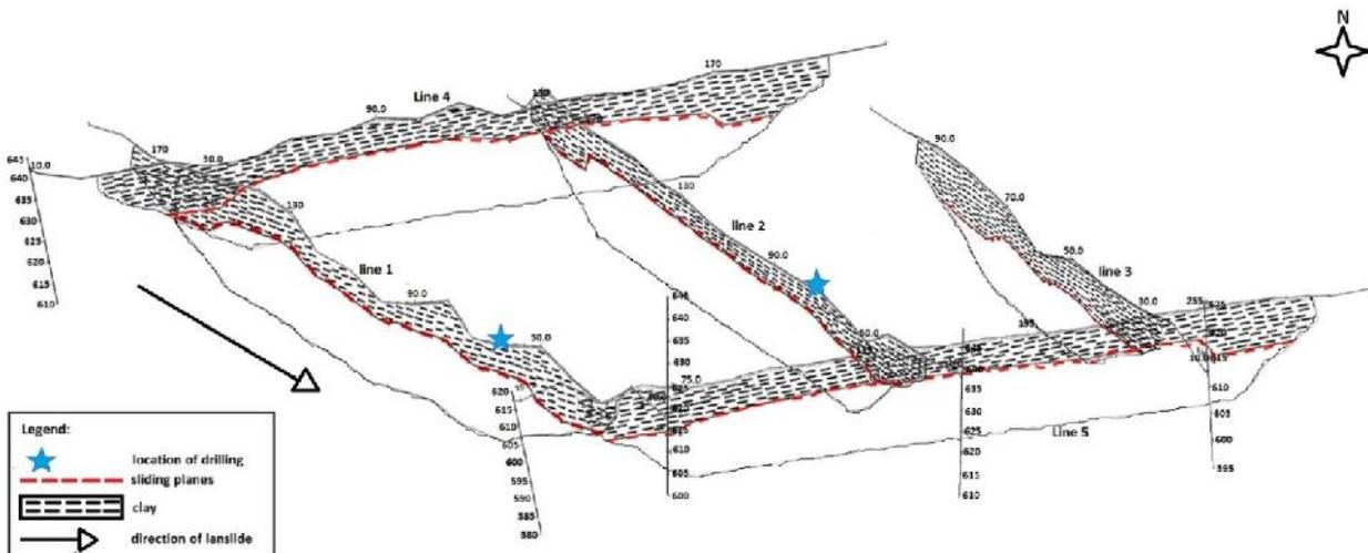
Fig12 . 2D Resistivity and Drilling Point Correlation
