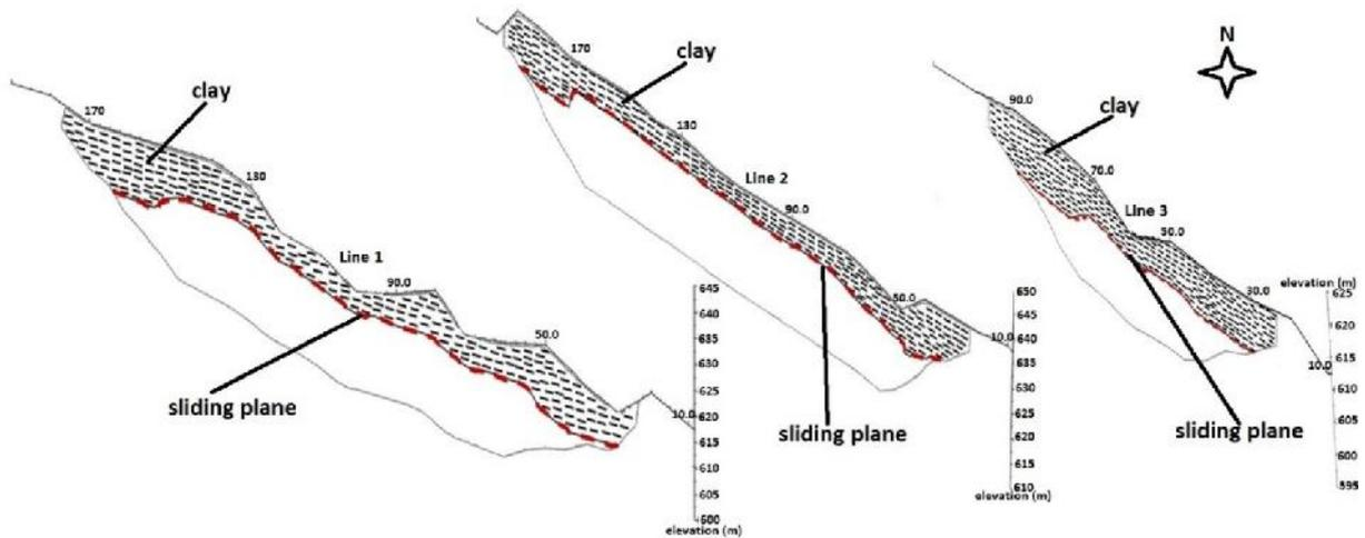
Fig 11. Correlation of 2D Resistivity Sections of Line 1, Line 2 and Line 3
