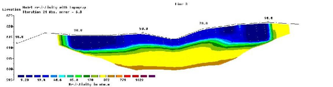
Fig 8. 2D Resistivity Line 3 (green line in fig 4)
