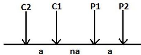
Fig. 3. Dipole-dipole configuration
