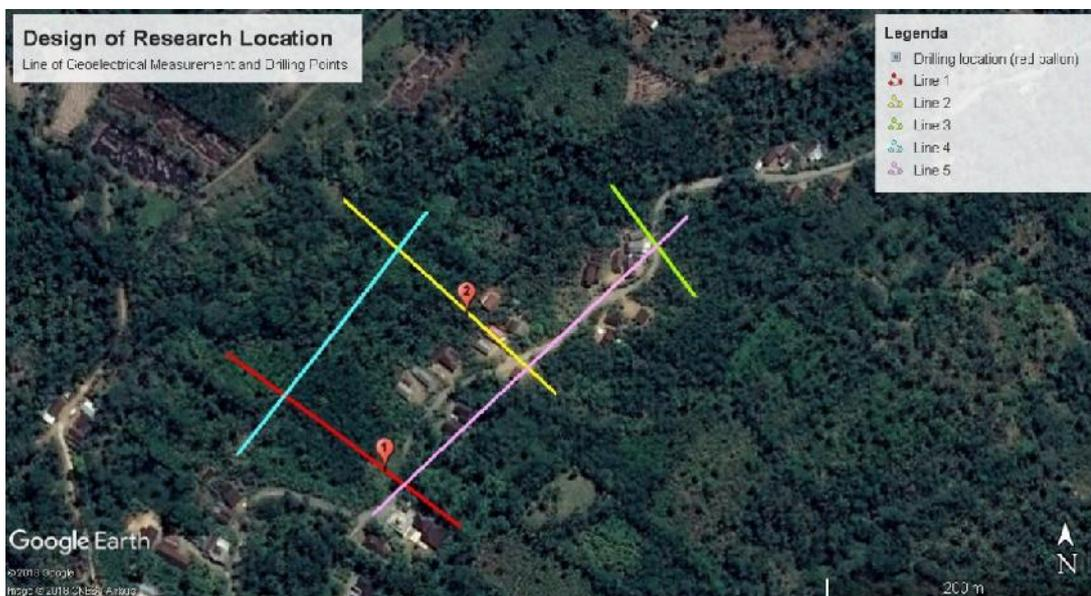
Fig 4. Geoelectric Resistivity Method Survey Measurement Design
