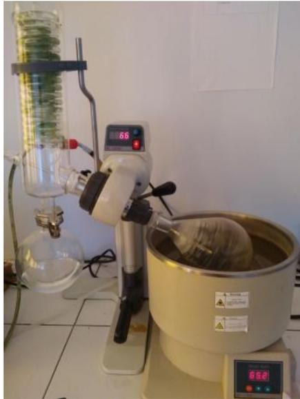
Gambar 2. 12 Proses Evaporator
